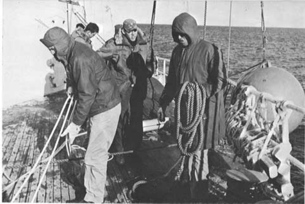
Buoy is held by whip while line is accurately measured and spliced to the current meters.
