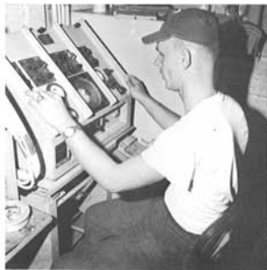
Pokela adjusts the fire control radar. Range to a contact can be read from the radar scope.
