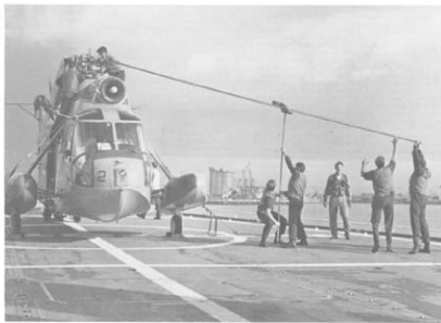
Top left: AEC Bradley releases the brakes prior to moving the helo. Bottom left: Flight crew prepares to tie down the helo after landing on deck. Bottom right: Folding the blades before moving the helo into the hanger.
